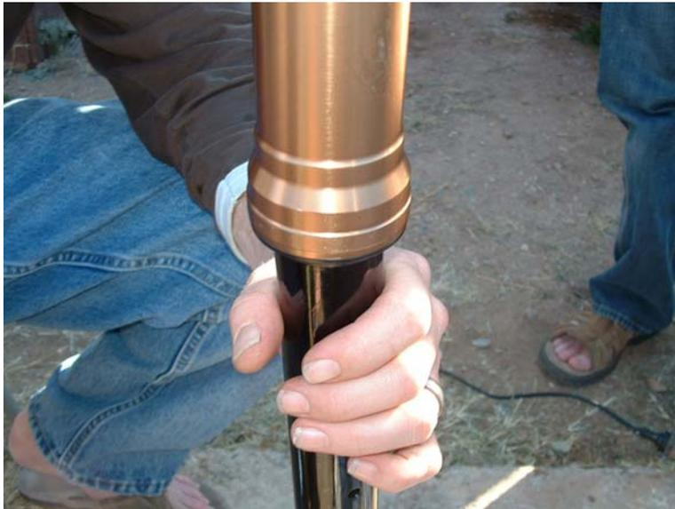
**Go ahead and fill with fork oil. Once full, pump the cartridge rod about 10 times, and then let sit a few minutes to ensure all air is out of the system. After that you triple check fluid level, and make sure its full.**
