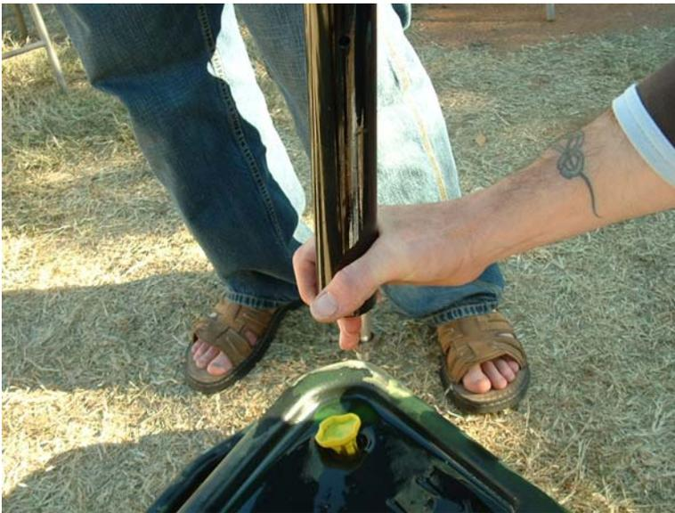
**Invert lower fork, holding cartridge rod to the side, and remove the 10mm hex head bolt. There is a copper washer on the bolt.**
