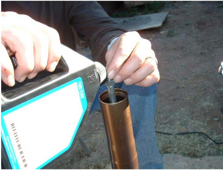
I used the Rebound adjustment rod to mark the 3.9" that the Busa requires the fork fluid to be at. Measurement is taken from the top, with the upper tube fully bottomed out on lower tube. Draw a mark at appropriate level.
