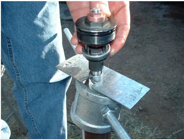
**Before final install of fork nut, measure to ensure there is 11mm of thread showing from end of the rod to top of nut. If not your adjustment range will be hindered. Also, loctite on the fork nut. Tighen fork nut while holding jam-nut.**
