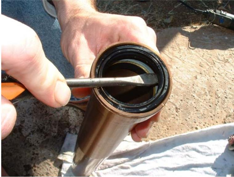
Seal seat, under the seal, just wipe it clean so you can inspect the inner race/bushing.
