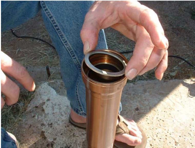
I used a Q-tip to clean the gasket area that the copper washer will seat, for the cartridge bolt.
