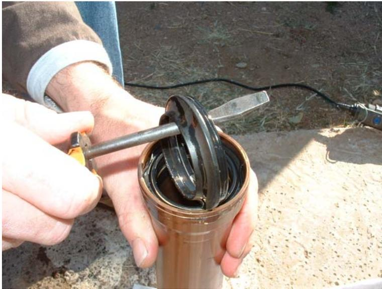
**Remove the Seal retainer spring. Simply pull one side out, and rotate around, it is a split ring fitted into a groove.**
