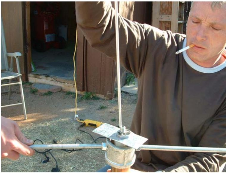
**Compress the spring again so you can remove the spacer-jam. It won't necessarily go shooting up out, but it will pop back up a little so keep control of the compressor tool.**
