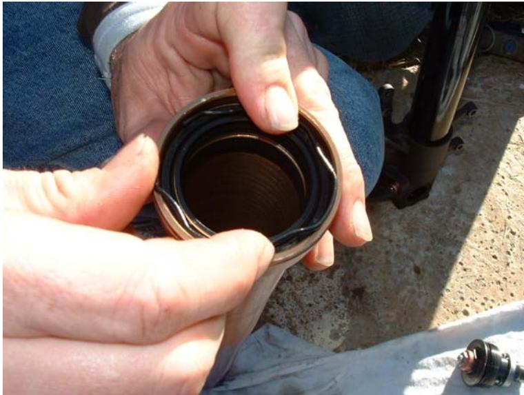
**Install Dust wiper, simply press into fully seated position.**
