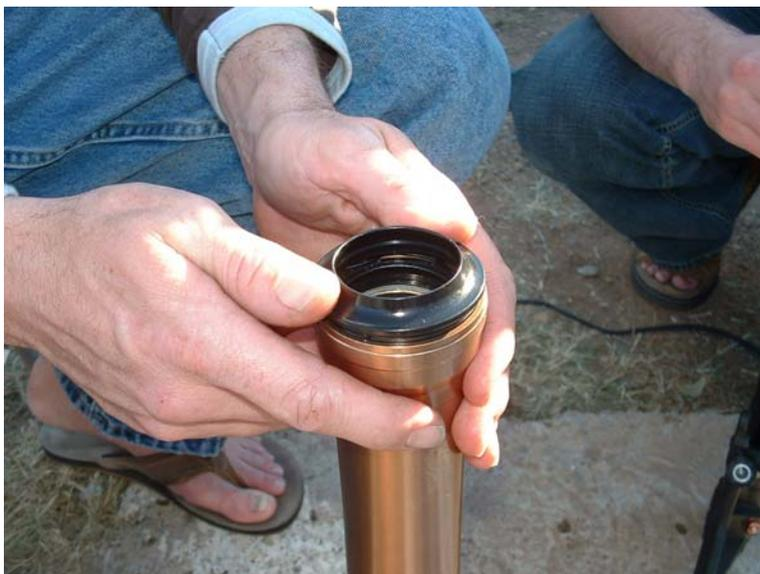
**Installed view, lube the wiper and seal inside surface to prevent seal damage during assembly.**
