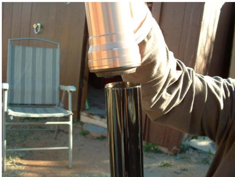
**Invert lower tube, grab the cartridge and pump a few times to finish draining as much old fork oil as possible.**
