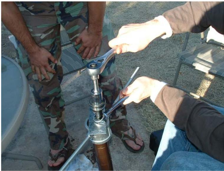
**Compress spring again to remove the plate. Let the spacer assembly ride up and engage the fork nut.**
