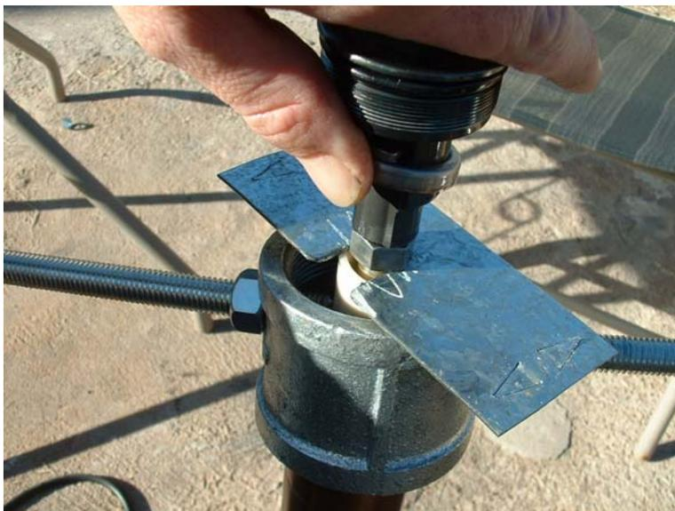
**17mm wrench on the jam-nut, and socket on the fork nut, loosen it up man!**
