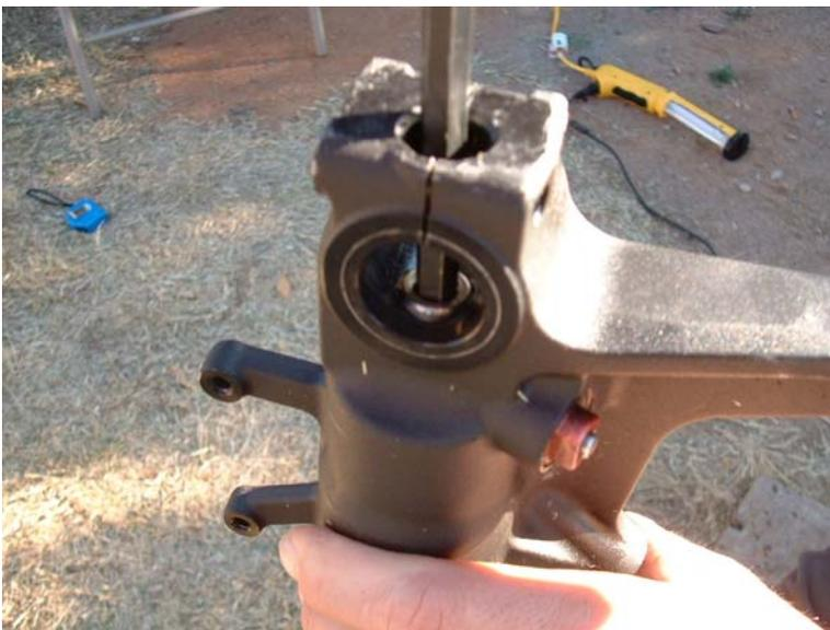
**Pull the cartridge out and pump to remove all oil.**
